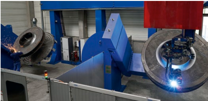
A five-axis robot arm enables efficiency in multiple welding stations
