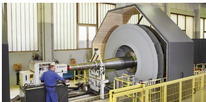
Balancing bench for rotor assemblies up to 5,000 mm diameter
