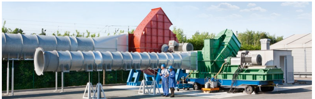
Performance test bench for centrifugal fans up to 1,000 kW at 400 V
