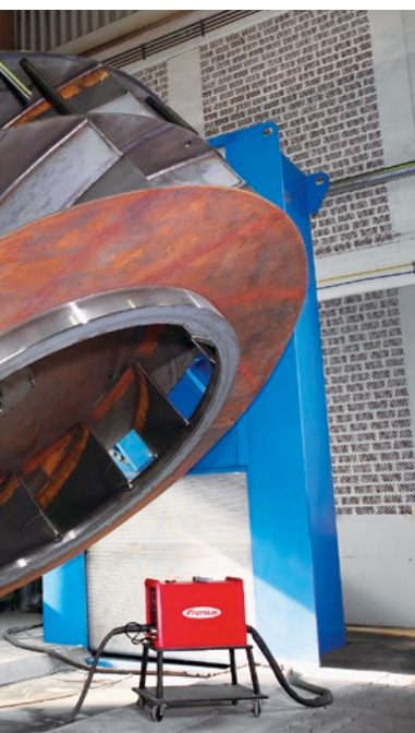
Positioner for safe and ergonomic welding of impellers
